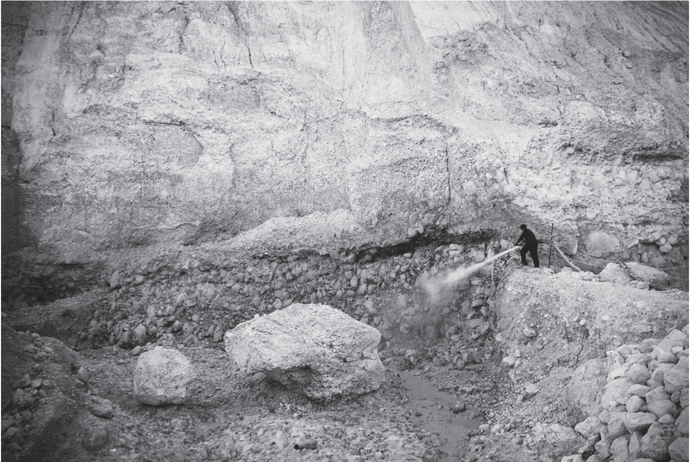
Venezuela: A diamond miner uses a high-pressure blast of water. Years of searching like this wears away the rock.
